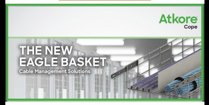
Cope Eagle Basket wire basket cable tray is a welded mesh cable management system produced from the highest quality steel wires. Eagle Basket's 2"x4" mesh permits continuous airflow to prevent heat buildup as well as dust and other contaminants. The Wire basket tray is produced by first welding a net, forming the channel, and then finishing after fabrication.
